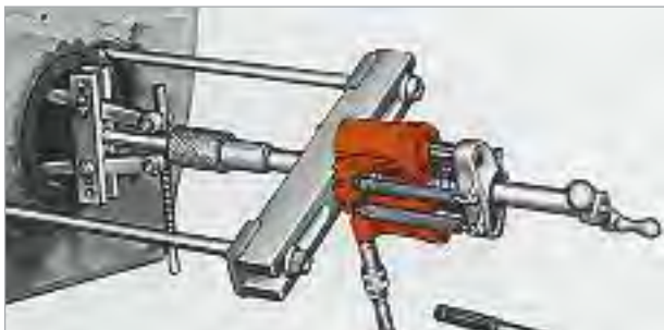
Combination of 50 ton capacity Push-Puller and cup pulling attachment simplifies the removal of a final drive axle seal.
