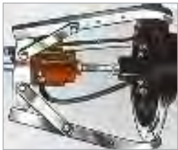
3-jaw puller provides grip while hydraulic hand pump provides power to push shaft from housing. Shaft protector is used on end of puller screw.
