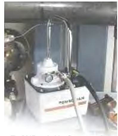
The PA17 used with a flange spreader
