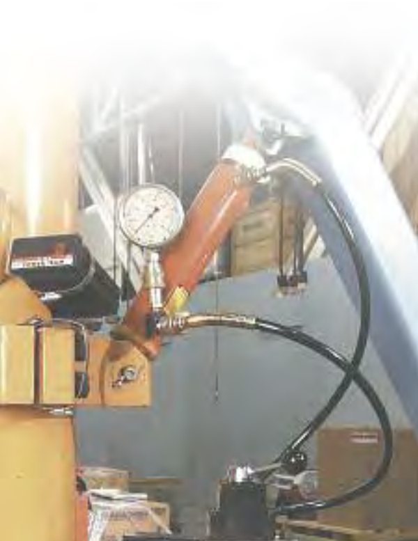
PA6D pump, DG100 digital pressure gauge and 25 ton cylinder used in a test fixture.
